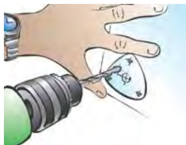
Drill hole for sensor wire.
